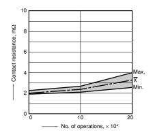
7-(2). Electrical life test (Lamp load) Sample: CA1a-12V-C, 3pcs. Load: 60Wx4, Inrush current: 110A, steady current: 20A Halogen lamp actual load Switching frequency: (ON:OFF = 1s:14s) Ambient temperature: Room temperature
