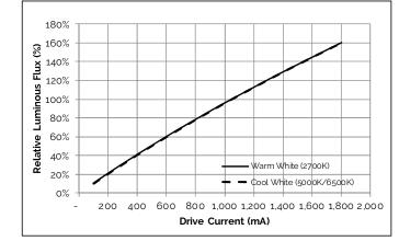
Figure 2: Relative Flux vs. Drive Current, T\_=25°C
