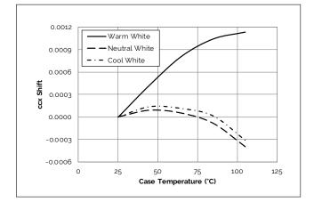
Figure 15: Typical ccx Shift vs. Case Temperature
