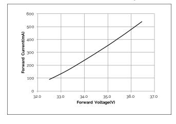
Figure 10: V10B Drive Current vs. Voltage (T<sub>c</sub>=25°C)
