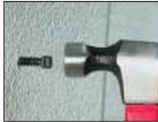
2. Hammer mount into hole.
