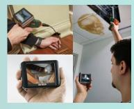
Extech's Video Borescope with a 5.2 mm diameter camera probe makes it possible to inspect hard to access areas through a small opening. It provides a glare-free close-up field of view.
