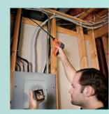
Extech's Video Borescope Inspection Camera with a 4.5mm camera provides a glare-free close-up field of view. It includes a 3.5" color TFT LCD wireless monitor that can be detached from the base and viewed from a remote location up to 32ft (9.75m) from measurement point. Images and videos can be captured with date/ time stamp and played back on the monitor
