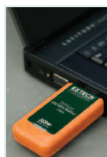
BRD10 - Optional Wireless USB Video Receiver allows user to stream live video to a PC and also can be remotely viewed via VOIP connection
