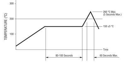
Processing Method: Reflow soldering with infrared heat or forced air convection (only once).
