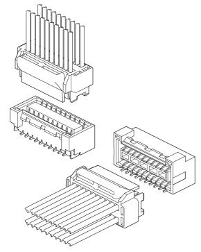
To meet the requirement of the high density mounting on PC board of flat panel TV, AV equipments etc., this connector is designed to the double-row type of 1.25mm pitch. Its operability is very well, in spite of the small size.
