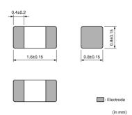
Chip ferrite beads for high frequency noise suppression over a wide frequency range.
