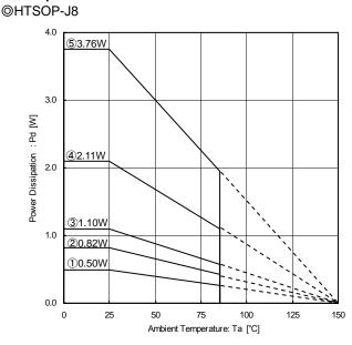
Measure condition: mounted on a ROHM board, and IC Substrate size: 70mm × 70mm × 1.6mm
