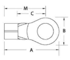
These non-insulated ring terminals are made of electrolytic copper for high conductivity. They can be installed with crimping tools having a single indentor or double indentor (recommended for solid wire). Serrated barrel increases grip on wire.
