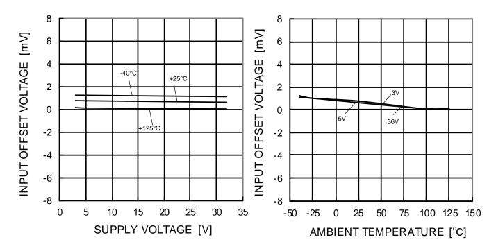
Figure 35. Input Offset Voltage vs Supply Voltage  $(V_{ICM}=0V, V_{OUT}=1.4V)$
