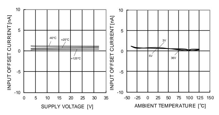
Figure 41. Input Offset Current vs Supply Voltage (V<sub>ICM</sub>=0V, V<sub>OUT</sub>=1.4V)
