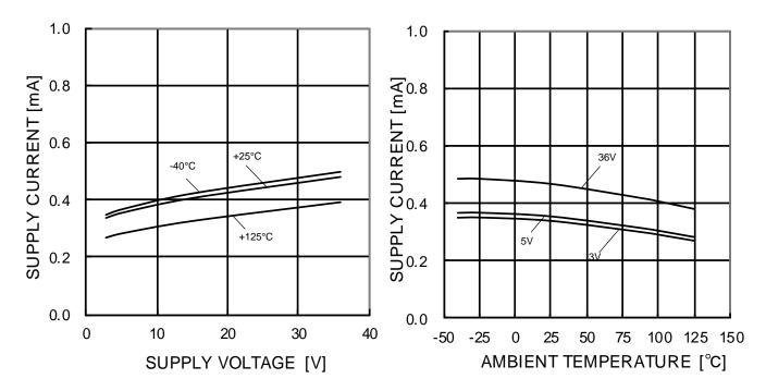
Figure 2. Supply Current vs Supply Voltage
