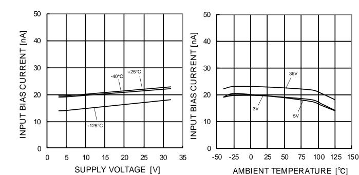
Figure 14. Input Bias Current vs Supply Voltage (V<sub>ICM</sub>=0V, V<sub>OUT</sub>=1.4V)
