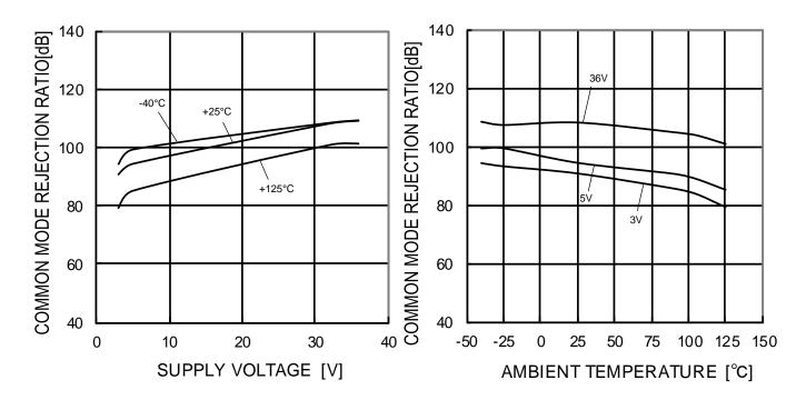
Figure 22. Common Mode Rejection Ratio vs Supply Voltage  $(V_{OUT}=1.4V)$
