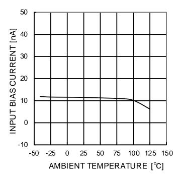
Figure 39. Input Bias Current vs Ambient Temperature (Vcc=30V, V<sub>ICM</sub>=28V, V<sub>OUT</sub>=1.4V)
