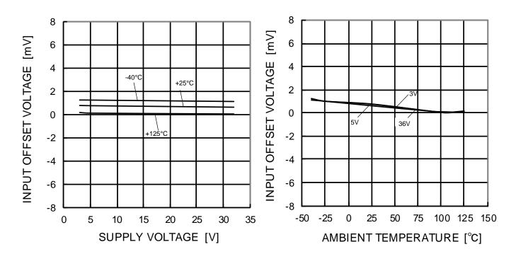
Figure 12. Input Offset Voltage vs Supply Voltage (V<sub>ICM</sub>=0V, V<sub>OUT</sub>=1.4V)
