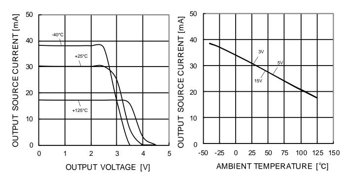
Figure 6. Output Source Current vs Output Voltage  $(V_{CC}=5V)$
