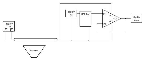
Figure 55. Measurement Circuit of EMI Evaluation
