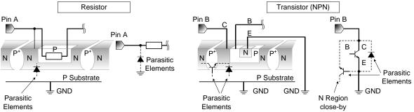
Figure 57. Example of monolithic IC structure
