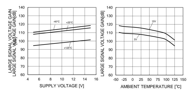
Figure 20. Large Signal Voltage Gain vs Supply Voltage  $(R_L=2k\Omega)$
