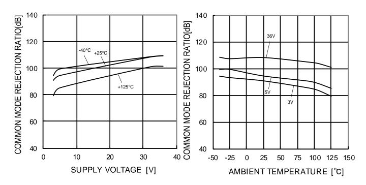
Figure 45. Common Mode Rejection Ratio vs Supply Voltage (Vout=1.4V)
