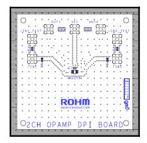
Figure 53. EMI Evaluation Board (BA82904Yxxx-C)
