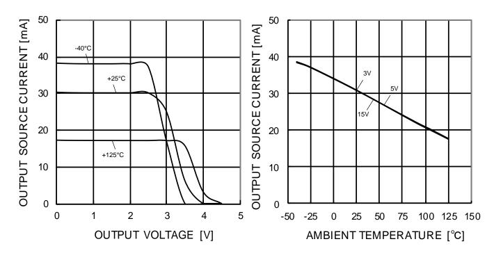
Figure 29. Output Source Current vs Output Voltage (Vcc=5V)
