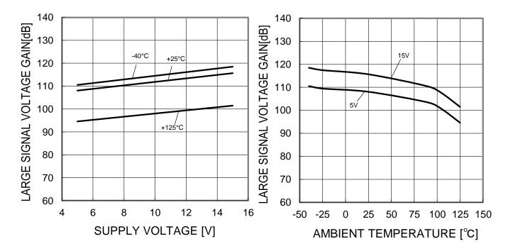
Figure 43. Large Signal Voltage Gain vs Supply Voltage  $(R_L=2k\Omega)$
