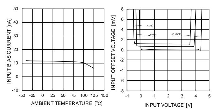
Figure 16. Input Bias Current vs Ambient Temperature  $(V_{CC}=30V, V_{ICM}=28V, V_{OUT}=1.4V)$
