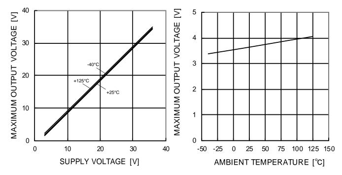
Figure 4. Maximum Output Voltage vs Supply Voltage  $(R_L=10k\Omega)$
