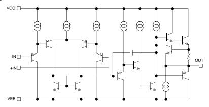
Figure 1. Simplified schematic (one channel only)
