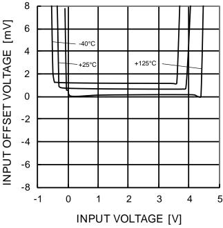
Figure 40. Input Offset Voltage vs Input Voltage (Vcc=5V)
