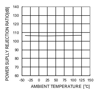
Figure 47. Power Supply Rejection Ratio vs Ambient Temperature
