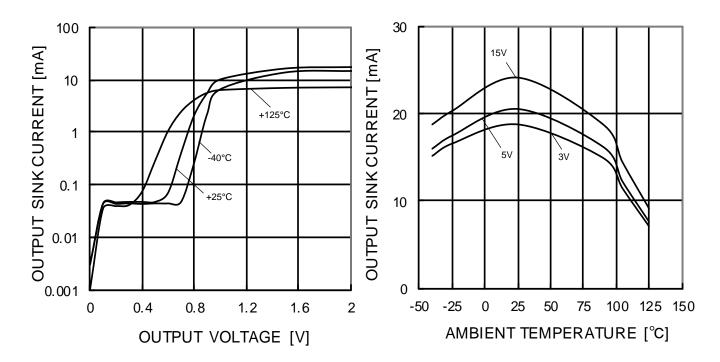
Figure 31. Output Sink Current vs Output Voltage  $(V_{CC}=5V)$
