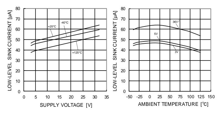
Figure 33. Low Level Sink Current vs Supply Voltage  $(V_{OUT}=0.2V)$
