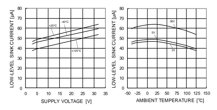
Figure 10. Low Level Sink Current vs Supply Voltage  $(V_{OUT}=0.2V)$
