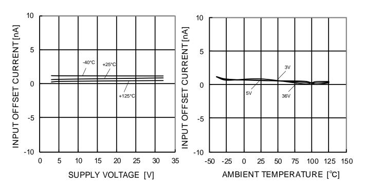
Figure 18. Input Offset Current vs Supply Voltage (V<sub>ICM</sub>=0V, V<sub>OUT</sub>=1.4V)
