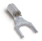
These non-insulated fork terminals are made of electrolytic copper for high conductivity. They can be installed with crimping tools having a single indentor or double indentor (recommended for solid wire). Serrated barrel increase grip on wire. Wire range identification is stamped on the tongue of each terminal.
