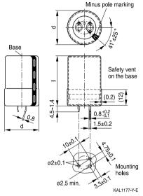
Snap-in capacitors are also available with 3 terminals (length 4.5-1.4 mm). PET insulation cap is positioned under the insulation sleeve.
