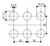
Dimensions of minimum space requirements (according to EN 50007 and IEC337-2C). Take to consideration the field of traverse of swing knobs (27mm) and the diameter of mushroom heads.
