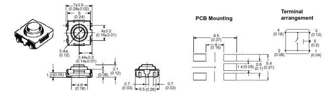
**Note:** Unless otherwise specified, a tolerance of  $\pm$  0.2 mm applies to all dimensions.
