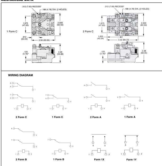
Dimensions in inches with metric equivalents in parentheses. Tolerance: ± .010"
