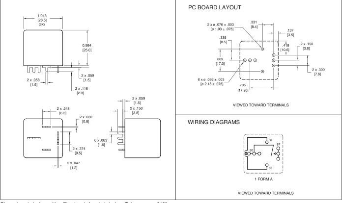
Dimensions in inches with millimeters in brackets below. Tolerance: ± .010"
