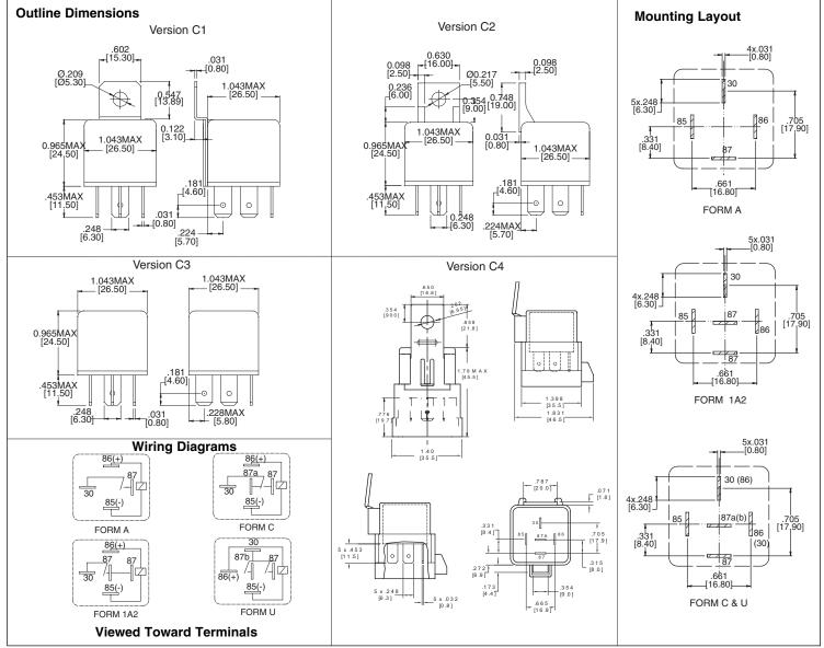
Dimensions in inches with metric equivalents in parentheses. Tolerance: ± .010"
