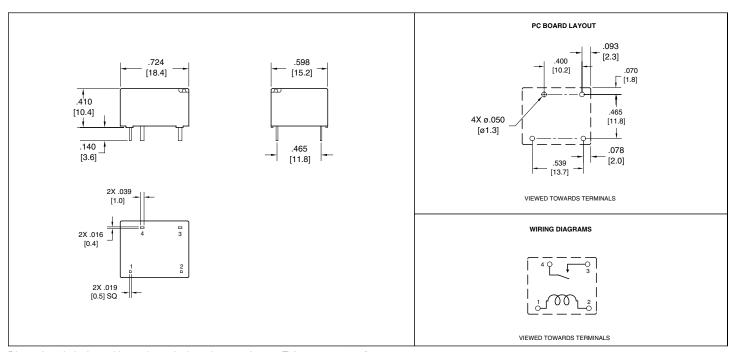
Dimensions in inches with metric equivalents in parentheses. Tolerance: ± .010"
