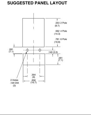
Dimensions in inches with metric equivalents in parentheses. Tolerance: ± .010"
