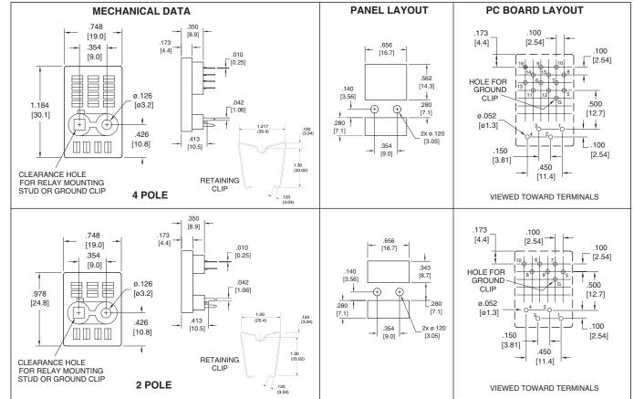
Dimensions in inches with metric equivalents in parentheses. Tolerance: ± .010"
