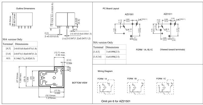
Dimensions in inches with metric equivalents in parentheses. Tolerance: ± .010"
