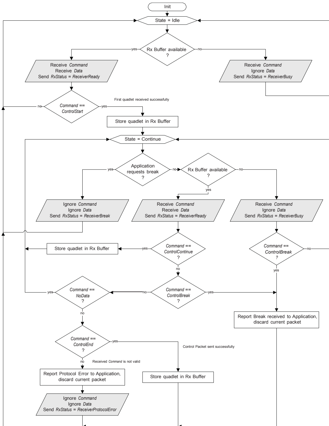
Figure 48-9. Control Packet Rx Device Protocol
