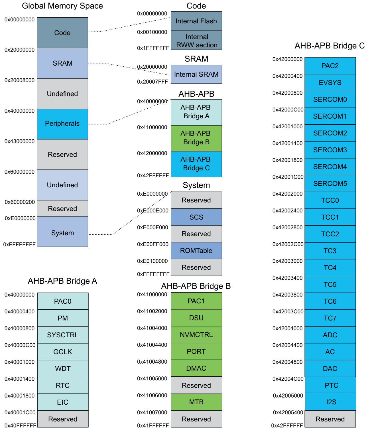
Figure 8-1. Atmel | SMART SAM DA1 Product Mapping
