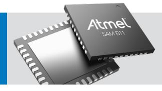
The Atmel<sup>®</sup> SmartConnect SAM B11 is an ultra-low-power Bluetooth<sup>®</sup> SMART (BLE 4.1) system on a chip (SoC) with integrated microcontroller (MCU), transceiver, modem, MAC, PA, TR switch, and power management unit (PMU). It is a standalone applications processor with 256KB of Flash memory and with embedded BLE connectivity.
