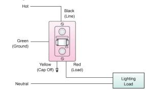
Adaptive Technology PIR Wall Switch AT1277 Series Wall Switches
