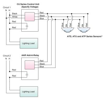
\*\*NOTE: For wiring sensors with isolated relay and photocell option (models with "RP" suffix): Photocell Option: Cap off Blue sensor wire. Connect Grey sensor wire to Blue control unit wire. Isolated Relay Option: Common-Blue/White wire, Normally Closed-Black/White wire, Normally Open-Yellow/White wire.
