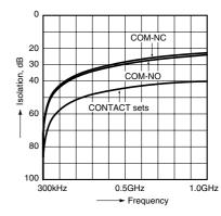
1-(2). High frequency characteristics (Impedance  $75\Omega$ )
