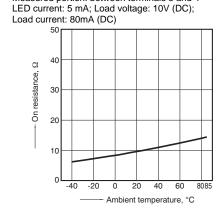
2. On resistance vs. ambient temperature
