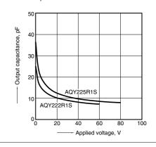
12.-(2) Output capacitance vs. applied voltage characteristics
