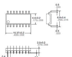
Terminal thickness = 0.15 .006 General tolerance: ±0.1 ±.004 mm inch
