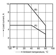
1.-(3) Load current vs. ambient temperature (AC output, 2 A type) Part No.: AQ2A2-ZP3/28VDC and AQ2A2-J-ZP3/28VDC
