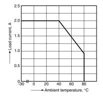
1.-(4) Load current vs. ambient temperature (AC output, 5 A type) Part No.: AQ5A2-ZP3/28VDC (A) When not using a heat sink
