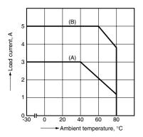
1.-(5) Load current vs. ambient temperature (DC output, 1 A and 2 A types) Part No.: AQ1AD2-3/28VDC and AQ2AD1-3/28VDC Allowable ambient temperature:
