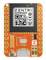
The AMW037-E01 evaluation board provides a quick and easy way to evaluate and develop using ZentriOS-Lite with the surface mounted <u>AMW307 module</u>. Using the AMW037 module is a breeze, simply plug the board into a computer using a standard USB cable, connect with a PC terminal application and start typing. The kit also comes with a fully licensed version of ZentriOS-Lite.
