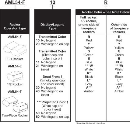
NOTE: AML54-F10 and AML54-F20 are one-piece, one-color full rockers. Thus only one color code letter is necessary when ordering. Include a two letter code for all other AML54-E (and AML54-T) catalog listings.
