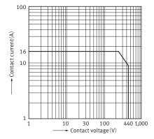
2. Max. switching power (DC resistive load)
