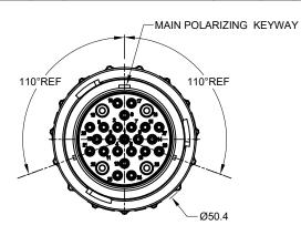
RECEP, 24:27 POS, SOCKET CONT., REDUCED DIA. SEAL, AHDP SERIES
