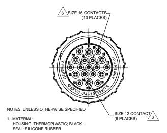
2. MODIFICATIONS: THREADED ADAPTER; REDUCED DIA. WIRE SEAL
