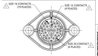
2. MODIFICATIONS: SMOOTH RING ADAPTER (SRA); REDUCED DIA. WIRE SEAL; SEALED PANEL MOUNT
