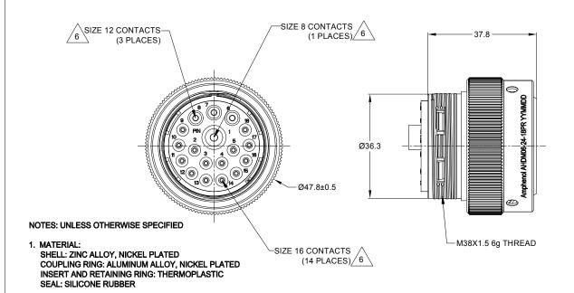
2. MODIFICATIONS: THREADED HOUSING; REDUCED DIA. WIRE SEAL
