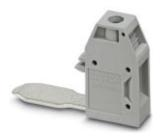
Pick-off terminal block, nom. voltage: 1000 V, nominal current: 57 A, connection method: Screw connection, number of connections: 1, cross section: 0.5 mm² - 10 mm², AWG: 20 - 8, width: 10.2 mm, height: 34.7 mm, color: gray, mounting type: on base element
