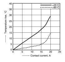
3. Coil temperature rise Sample: ADJ56024, 6 pcs. Coil applied voltage: 100 %V, 130 %V of rating Contact current: 0 A, 10 A Measured portion: Inside the coil, Ambient temperature: Room temperature, 70°C 158°F
