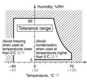
• Atmospheric pressure: 86 to 106 kPa Temperature and humidity range for usage, transport, and storage
