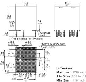
Tolerance Max. 1mm .039 inch: ±0.1 ±.004 1 to 3mm .039 to .118 inch: ±0.2 ±.008 ±0.3 ±.012
