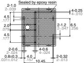
Dimension: Tolerance Max. 1mm .039 inch: ±0.1 ±.004
