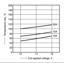
1-(5). Coil temperature rise (at room temperature)
