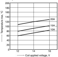
1-(6). Coil temperature rise (at 85°C 185°F) Sample: ACJ5212, 3pcs Measured portion: Inside the coil Contact carrying current: 10A, 15A, 20A Ambient temperature: 85°C 185°F
