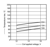
1-(3). Coil temperature rise (at room temperature)
