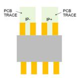
When the connection to the input pin covers only the horizontal portion of the input pin, there is a sensitivity variation of about +1.2% versus the recommended PCB trace layout (as shown in Figure 15).
