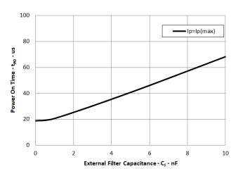
Figure 10: Rise Time vs. External Filter
