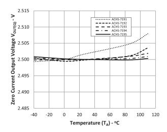
Figure 3: Nonlinearity vs. Temperature
