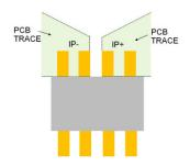
When the connection to the input pin covers only the vertical portion of the input pin, there is a sensitivity variation of about –0.6% versus the recommended PCB trace layout as shown in Figure 14.
