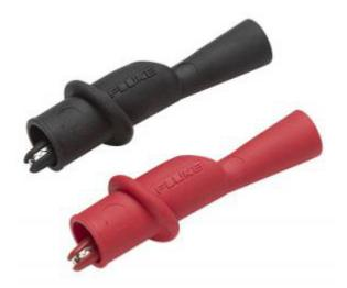
Slide-on alligator clips (red, black) compatible with TL71, TL75, TL175 and TP175. Insulated alligator clip jaws provide 8 mm opening with flexible boots. CAT III 1000 V, CAT IV 600 V, 10 A rating. One year warranty.
