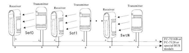
Note: it is possible for transmitter not to connect the bue wire, but if in this case, it will not display the strength of signal, and can not adjust the transmitting frequency automatically according to signal strength.
