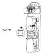
2.Adjust the vertical and horizontal optic axis following the picture below in order to get a best signal strength. If the signal is less than 1.8, please adjust again to get a better signal strength.
