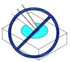
3. Do not stack together assembled PCBs containing exposed LEDs. Impact may scratch the silicone lens or damage the internal circuitry.
