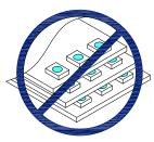
4.1. The outer diameter of the SMD pickup nozzle should not exceed the size of the LED to prevent air leaks. The inner diameter of the nozzle should be as large as possible.
