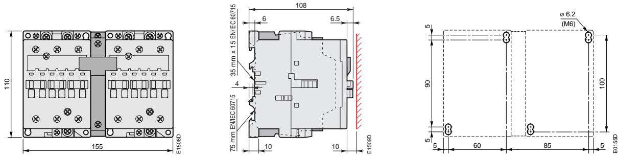
A 50, A 63, A 75, AF 50, AF 63, AF 75 + VE 5-2 electrical and mechanical interlock unit
