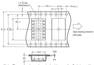
Note: The perforations along both sides are for Switches with 7 poles or more. The perforations on the bottom of the diagram are not provided on Switches with 6 poles or less.
