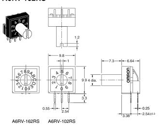
Note: A tolerance of ±0.4 mm applies to the above dimensions unless otherwise specified.
